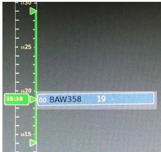
Figure 3: Example of a “Slot Zone” displayed on iAMAN in green (here around BAW358 that has 19 mins of ATFCM delays)
